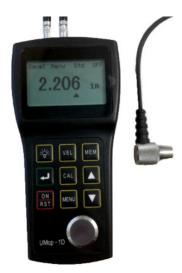
Ultrasonic thickness gauges measure the thickness of ultrasonic wave well-conductive materials with parallel top and bottom surfaces. It measures the thickness of both metal (steel, aluminum, titanium, etc.) and nonmetal (plastics, ceramics, glass, etc.) parts. They are commonly used to measure (remaining) wall thickness of pipes and pressure vessels.
